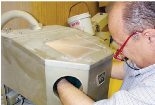
While abrasive blasting dental castings, a worker uses an enclosure that isolates silica dust.
